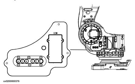
Internal brake release unit with push buttons, located on the robot frame
