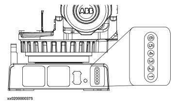
Internal brake release unit with push buttons, located on the robot base
